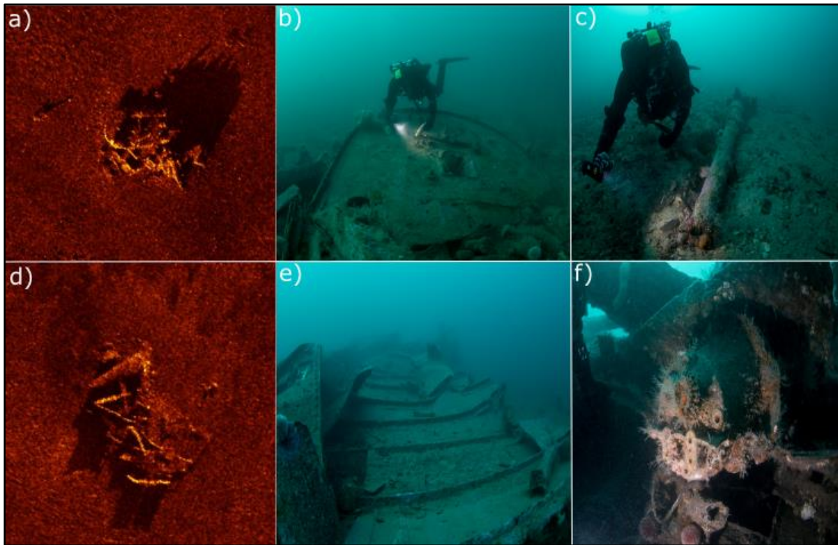
Plate 14 a) side scan sonar image SS070 & SS069 b) SS069 searchlight platform c) SS070 8.8cm L/45 gun d) side scan sonar image SS071 e) SS071 searchlight platform f) SS071 in-situ searchlight controller
