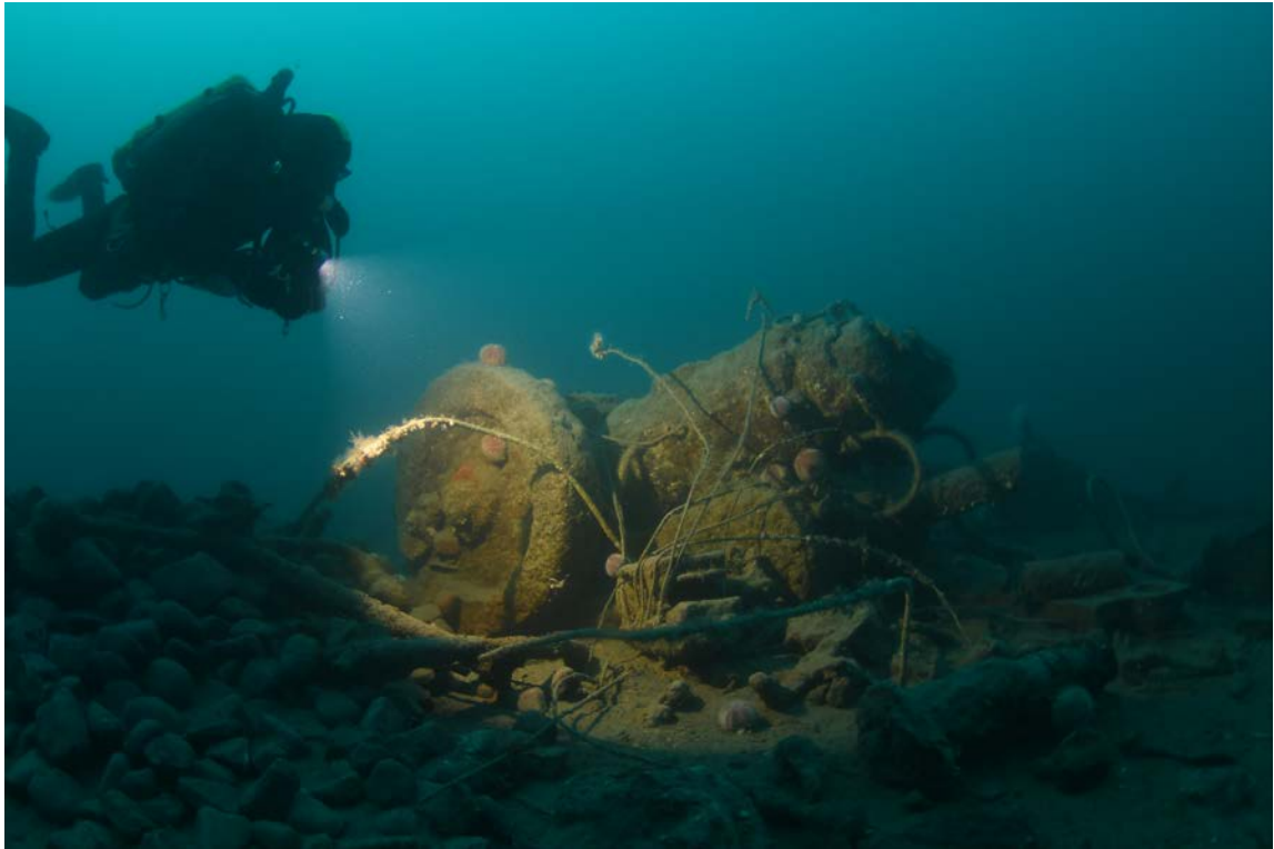
Figure 8: Two-cylinder engine with large fly-wheel on forward end. Start of ballast pile to left of image.
