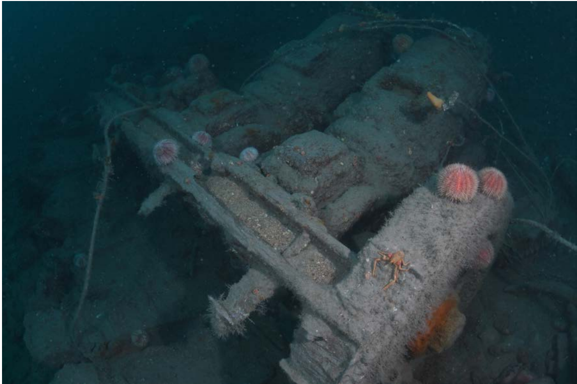
Figure 10: Close up of engine showing two cylinders, flywheel and mounting frame. The engine had fallen to port, exposing the concrete ballast below (left of image).
