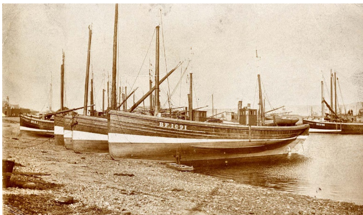
Figure: 27. A converted Zulu of the same style as Edindoune showing the capstan forward and new wheelhouse. (Glenn McIntosh).
