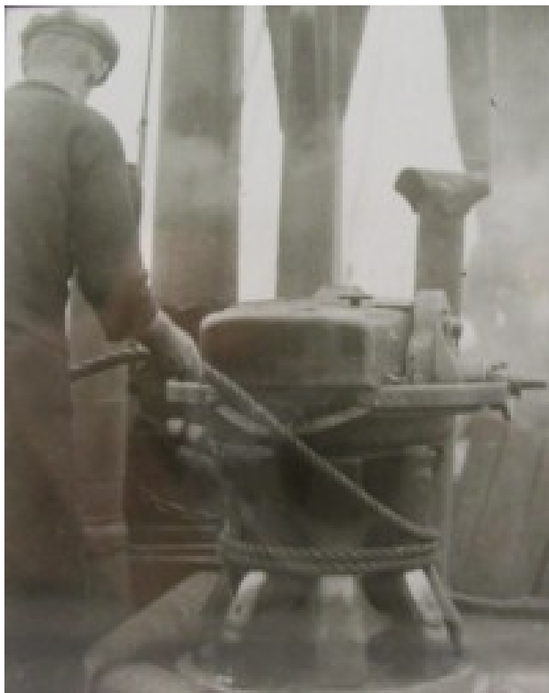
Figure 30: Deck capstan on a herring drifter with funnel behind (left). Typical arrangement of steam powered capstan showing the vertically mounted boiler below deck (right).
