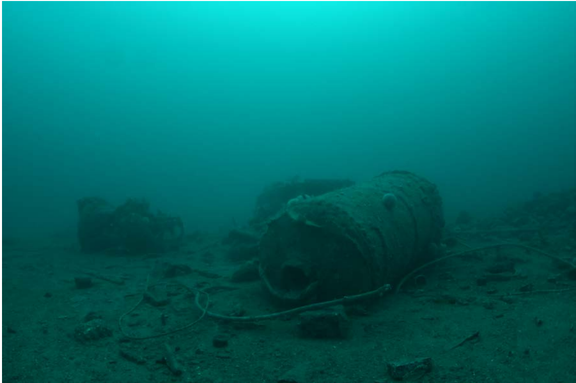
Figure 18: Group of objects lying forward of the ballast pile (visible to right of image), including a boiler (foremost), capstan winch (to left), mast step and anchor chain (rear of group).
